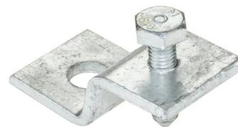
**Technical:****Product Type** Beam Clamp**Weight** 0.15 Kgs**Gauge** 6mm**Material** Post Hot-Dipped Galvanised (HDG)**Colour/Finish** Self Colour**Standards** BS 6946:1988**Supplied With** Cone pointed screw (TF050) supplied.
