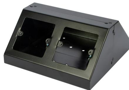
**Technical:****Product Type** Pedestal Boxes**Width** 190mm**Depth** 180mm**Height** 90mm**Weight** 0.70 Kgs**Dimensions** Overall Size: (D) 180mm x (W) 190mm X (H) 90mm**Angle** 45°**Number of Gangs** 2 x 1**Gauge** 1.0mm**Material** Pre-Galvanised Steel (Zinc Coated)**Colour/Finish** Black (RAL 9005)**Supplied With** 1 x 20mm knockout 1 x 25mm knockout Earth terminal in base
