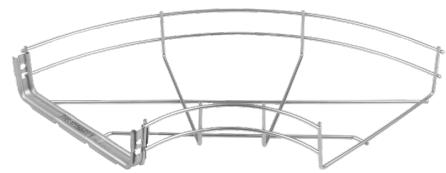
**Technical:****Product Type** Pre-Fabricated Bend**Width** 200mm**Height** 60mm**Weight** 0.37 Kgs**Angle** 90°**Material** Pre-Galvanised Steel (Zinc Coated)**Colour/Finish** Self Colour**Supplied With** Pre-Installed FastConnect Coupler
