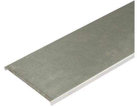
**Technical:****Product Type** Basket Tray Lid**Width** 200mm**Height** 10mm**Length** 3000mm**Weight** 6.78 Kgs**Material** Pre-Galvanised Steel (Zinc Coated)**Colour/Finish** Self Colour
