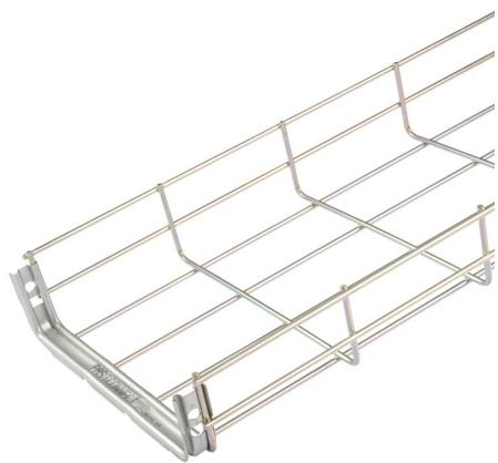
**Technical:****Product Type** Basket Tray**Width** 200mm**Height** 60mm**Length** 3000mm**Weight** 2.73 Kgs**Dimensions** 200 x 60mm mesh**Diameter** 3.9mm (Steel wire frame)**Outside Diameter** 3.9mm (Steel wire frame)**Material** Electro Zinc (E.Z)**Colour/Finish** Self Colour**Standards** BS EN 61537:2007**Supplied With** Pre-Installed FastConnect Coupler
