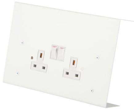
**Technical:****Product Type** Plates**Depth** 60mm**Height** 200mm**Weight** 1.07 Kgs**Number of Gangs** 2**Gauge** 1.0mm**Material** Pre-Galvanised Steel (Zinc Coated)**Colour/Finish** White (RAL 9016)**Standards** BS EN 10346:2015**Compliance** Category 6a**Supplied With** Bridge and Fixing Screws**Pack Quantity** Each**Important:**
