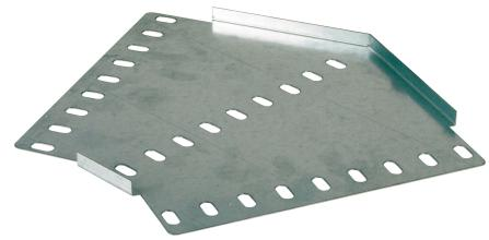
**Technical:****Product Type** Flat Bend**Width** 225mm**Height** 10mm**Weight** 0.77 Kgs**Angle** 45°**Gauge** Light Duty**Material** Pre-Galvanised Steel (Zinc Coated)**Colour/Finish** Self Colour**Standards** BS EN 61537:2007; BS EN 10346:2015**Pack Quantity** 1
