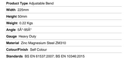
The approximate weights given are for pre-galvanised finish only, in kilograms (nominal) and subject to material thickness tolerance.
