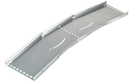
**Technical:****Product Type** Adjustable Bend**Width** 225mm**Height** 25mm**Weight** 1.00 Kgs**Angle** 5°-95°**Gauge** Medium Duty**Material** Zinc Magnesium Steel ZM310**Colour/Finish** Self Colour**Standards** BS EN 61537:2007; BS EN 10346:2015
