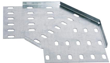
**Technical:****Product Type** Flat Bend**Width** 225mm**Height** 10mm**Weight** 0.77 Kgs**Angle** 90°**Gauge** Light Duty**Material** Zinc Magnesium Steel ZM310**Colour/Finish** Self Colour**Standards** BS EN 61537:2007; BS EN 10346:2015**Pack Quantity** 1
