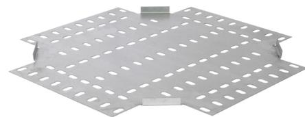
**Technical:****Product Type** Flat Fourway**Width** 225mm**Height** 10mm**Weight** 0.92 Kgs**Gauge** Light Duty**Material** Zinc Magnesium Steel ZM310**Colour/Finish** Self Colour**Standards** BS EN 61537:2007; BS EN 10346:2015**Pack Quantity** 1
