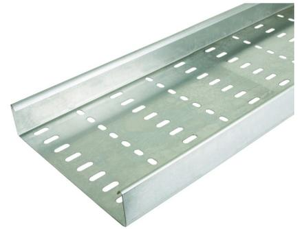
**Technical:****Product Type** Cable Tray**Width** 225mm**Height** 50mm**Length** 3000mm**Weight** 7.32 Kgs**Gauge** Heavy Duty**Material** Pre-Galvanised Steel (Zinc Coated)**Colour/Finish** Self Colour**Standards** BS EN 61537:2007; BS EN 10346:2015
