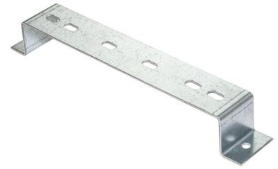
**Technical:****Product Type** Stand Off Bracket**Width** 225mm**Height** 40mm**Weight** 0.21 Kgs**Material** Pre-Galvanised Steel (Zinc Coated)**Colour/Finish** Self Colour**Standards** BS EN 10346:2015
