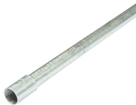
**Technical:****Product Type** Class 4 Conduit**Length** 3750mm**Weight** 2.81 Kgs**Diameter** 25mm**Outside Diameter** Min 24.60 - Max 25.00**Gauge** 1.6mm +- 0.15**Material** Post Hot-Dipped Galvanised (HDG)**Colour/Finish** Self Colour**Standards** BS EN 61386-1:2008+A1:2018**Supplied With** Threaded ends with one end fitted with coupler**Pack Quantity** 30 Metres (8 Lengths)**No of Lengths Per Bundle** 8
