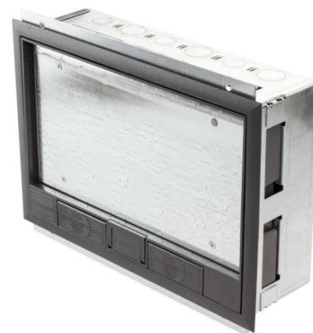
**Technical:****Product Type** Cavity Floor Box**Width** 225mm**Depth** 87mm**Length** 320mm**Weight** 2.60 Kgs**Dimensions** Overall Size: (L) 320mm x (W) 225mm Floor Cut-Out Size: (L) 305mm x (W) 205mm**Number of Compartments****Material** Pre-Galvanised Steel (Zinc Coated) / Polycarbonate**Colour/Finish** Self Colour**Supplied With** 20mm / 25mm Knockouts**Extra Information**
