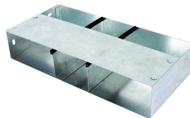
**Technical:****Product Type** Flush Screed Floor Trunking**Width** 350mm**Weight** 0.85 Kgs**Number of Compartments****Material** Pre-Galvanised Steel (Zinc Coated)**Colour/Finish** Self Colour**Standards** BS EN 10346:2015**Important:**
