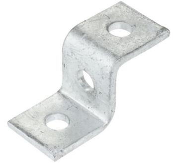
**Technical:****Product Type** Bracket**Height** 40mm**Weight** 0.19 Kgs**Gauge** 6mm**Material** Post Hot-Dipped Galvanised (HDG)**Colour/Finish** Self Colour**Standards** BS 6946:1988
