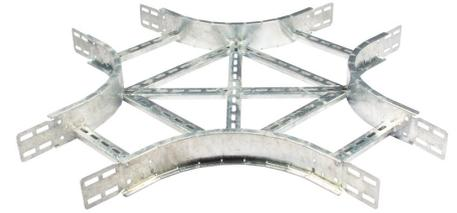
**Technical:****Product Type** Fourway**Width** 300mm**Height** 100mm**Weight** 9.40 Kgs**Diameter** 300mm Radius**Gauge** 1.5mm**Material** Post Hot-Dipped Galvanised (HDG)**Colour/Finish** Self Colour**Standards** BS EN ISO 1461:2009
