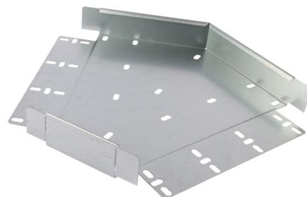
**Technical:****Product Type** Flat Bend**Width** 300mm**Height** 50mm**Weight** 1.44 Kgs**Angle** 45°**Gauge** Heavy Duty**Material** Pre-Galvanised Steel (Zinc Coated)**Colour/Finish** Self Colour**Standards** BS EN 61537:2007; BS EN 10346:2015
