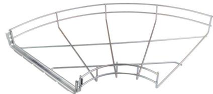
**Technical:****Product Type** Pre-Fabricated Bend**Width** 300mm**Height** 60mm**Weight** 0.64 Kgs**Angle** 90°**Material** Pre-Galvanised Steel (Zinc Coated)**Colour/Finish** Self Colour**Supplied With** Pre-Installed FastConnect Coupler
