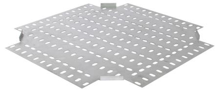
**Technical:****Product Type** Flat Fourway**Width** 300mm**Height** 10mm**Weight** 1.97 Kgs**Gauge** Light Duty**Material** Pre-Galvanised Steel (Zinc Coated)**Colour/Finish** Self Colour**Standards** BS EN 61537:2007; BS EN 10346:2015**Pack Quantity** 1
