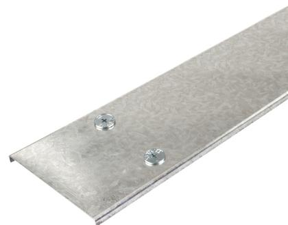
**Technical:****Product Type** Lid**Width** 300mm**Height** 10mm**Length** 3000mm**Material** Pre-Galvanised Steel (Zinc Coated)**Colour/Finish** Self Colour**Standards** BS EN 50085-2-1 2006; BS EN 10346:2015**Supplied With** Turnbuckle lid fixings
