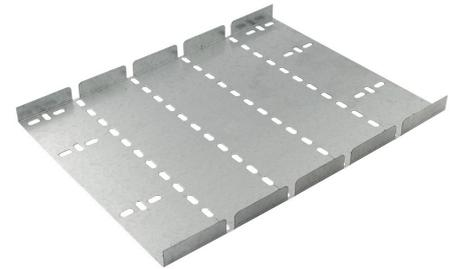
**Technical:****Product Type** Universal Riser**Width** 300mm**Height** 25mm**Weight** 0.99 Kgs**Gauge** Medium Duty**Material** Zinc Magnesium Steel ZM310**Colour/Finish** Self Colour**Standards** BS EN 61537:2007; BS EN 10346:2015
