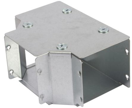
**IMAGE FOR ILLUSTRATIVE PURPOSES ONLY****Technical:****Product Type** Gusset Tee**Width** 300mm**Height** 150mm**Number of Compartments****Material** Pre-Galvanised Steel (Zinc Coated)**Colour/Finish** Self Colour**Standards** BS EN 50085-2-1 2006; BS EN 10346:2015
