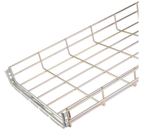
**Technical:****Product Type** Basket Tray**Width** 300mm**Height** 60mm**Length** 3000mm**Weight** 4.47 Kgs**Dimensions** 300 x 60mm mesh**Diameter** 4.4mm (Steel wire frame)**Outside Diameter** 4.4mm (Steel wire frame)**Material** Electro Zinc (E.Z)**Colour/Finish** Self Colour**Standards** BS EN 61537:2007**Supplied With** Pre-Installed FastConnect Coupler
