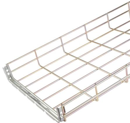
**Technical:****Product Type** Basket Tray**Width** 300mm**Height** 60mm**Length** 3000mm**Weight** 4.47 Kgs**Dimensions** 300 x 60mm mesh**Diameter** 4.4mm (Steel wire frame)**Outside Diameter** 4.4mm (Steel wire frame)**Material** Electro Zinc (E.Z)**Colour/Finish** Self Colour**Standards** BS EN 61537:2007**Supplied With** Pre-Installed FastConnect Coupler
