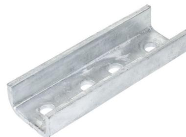
**Technical:****Product Type** Coupler**Width** 41mm**Height** 21mm**Weight** 0.50 Kgs**Gauge** 6mm**Material** Post Hot-Dipped Galvanised (HDG)**Colour/Finish** Self Colour**Standards** BS 6946:1988
