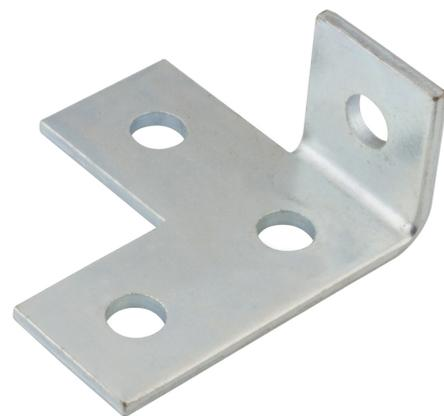
**Technical:****Product Type** Bracket**Weight** 0.29 Kgs**Angle** 90°**Gauge** 6mm**Material** Post Hot-Dipped Galvanised (HDG)**Colour/Finish** Self Colour**Standards** BS 6946:1988
