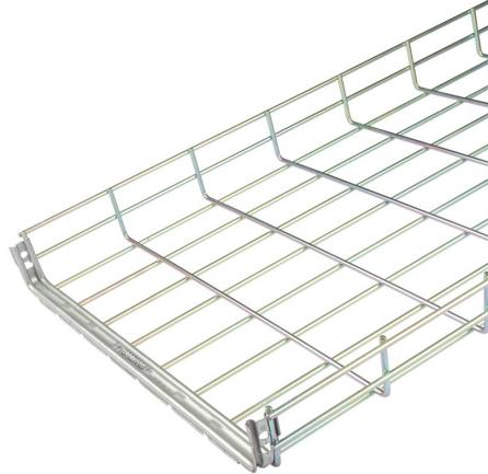
**Technical:****Product Type** Basket Tray**Width** 400mm**Height** 60mm**Length** 3000mm**Weight** 6.51 Kgs**Dimensions** 400 x 60mm mesh**Diameter** 4.8mm (Steel wire frame)**Outside Diameter** 4.8mm (Steel wire frame)**Material** Electro Zinc (E.Z)**Colour/Finish** Self Colour**Standards** BS EN 61537:2007**Supplied With** Pre-Installed FastConnect Coupler
