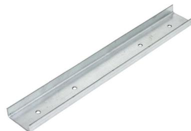
**Technical:****Product Type** Coupler**Width** 41mm**Height** 21mm**Weight** 0.20 Kgs**Material** Pre-Galvanised Steel (Zinc Coated)**Colour/Finish** Self Colour**Standards** BS 6946:1988**Supplied With** 4x M6 Screws
