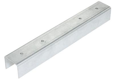
**Technical:****Product Type** Coupler**Width** 41mm**Height** 41mm**Weight** 0.35 Kgs**Material** Pre-Galvanised Steel (Zinc Coated)**Colour/Finish** Self Colour**Standards** BS 6946:1988**Supplied With** 4x M6 Screws
