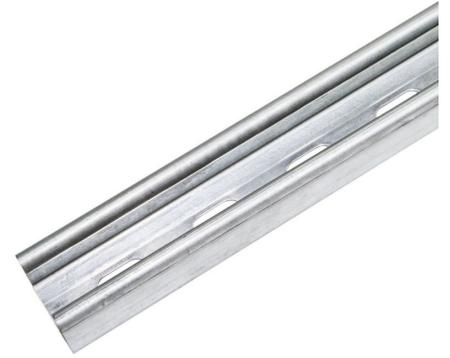
**Technical:****Product Type** Strut Channel**Width** 41mm**Height** 41mm**Length** 3000mm**Weight** 5.94 Kgs**Gauge** 2.5mm**Material** Pre-Galvanised Steel (Zinc Coated)**Colour/Finish** Self Colour**Standards** BS 6946:1988
