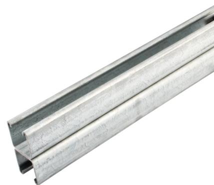
**Technical:****Product Type** Strut Channel**Width** 41mm**Height** 82mm**Length** 3000mm**Weight** 11.88 Kgs**Gauge** 2.5mm**Material** Zinc Magnesium Steel ZM310**Colour/Finish** Self Colour**Standards** BS 6946:1988
