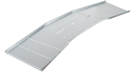
**Technical:****Product Type** Adjustable Bend**Width** 450mm**Height** 25mm**Weight** 1.60 Kgs**Angle** 5°-95°**Gauge** Medium Duty**Material** Zinc Magnesium Steel ZM310**Colour/Finish** Self Colour**Standards** BS EN 61537:2007; BS EN 10346:2015
