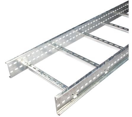
**Technical:****Product Type** Ladder Tray**Width** 450mm**Height** 125mm**Length** 3000mm**Weight** 16.30 Kgs**Dimensions** 300mm Rung Pitch**Gauge** 1.5mm**Material** Post Hot-Dipped Galvanised (HDG)**Colour/Finish** Self Colour**Standards** BS EN ISO 1461:2009**Extra Information**
