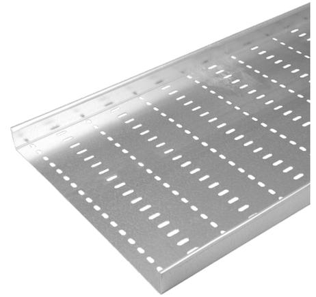
**Technical:****Product Type** Cable Tray**Width** 450mm**Height** 50mm**Length** 3000mm**Weight** 12.09 Kgs**Gauge** Heavy Duty**Material** Pre-Galvanised Steel (Zinc Coated)**Colour/Finish** Self Colour**Standards** BS EN 61537:2007; BS EN 10346:2015
