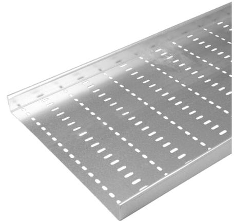
**Technical:****Product Type** Cable Tray**Width** 450mm**Height** 50mm**Length** 3000mm**Weight** 12.09 Kgs**Gauge** Heavy Duty**Material** Zinc Magnesium Steel ZM310**Colour/Finish** Self Colour**Standards** BS EN 61537:2007; BS EN 10346:2015
