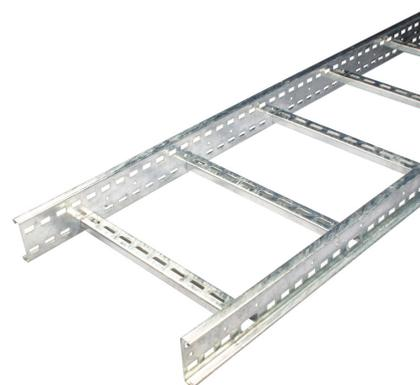
**Technical:****Product Type** Ladder Tray**Width** 450mm**Height** 100mm**Length** 3000mm**Weight** 14.60 Kgs**Dimensions** 300mm Rung Pitch**Gauge** 1.5mm**Material** Post Hot-Dipped Galvanised (HDG)**Colour/Finish** Self Colour**Standards** BS EN ISO 1461:2009**Important:**
