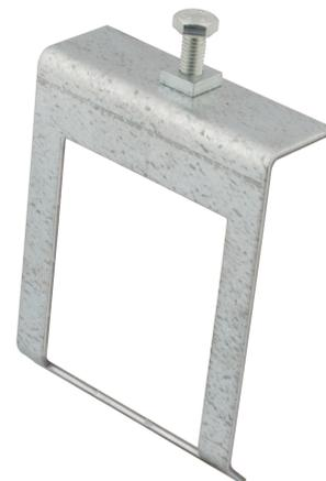
**Technical:****Product Type** Beam Clamp**Width** 50mm**Height** 50mm**Weight** 0.12 Kgs**Material** Pre-Galvanised Steel (Zinc Coated)**Colour/Finish** Self Colour**Standards** BS EN 10346:2015**Important:**
