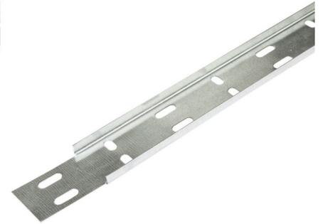
**Technical:****Product Type** Cable Tray**Width** 50mm**Height** 10mm**Length** 3000mm**Weight** 1.35 Kgs**Gauge** Light Duty**Material** Pre-Galvanised Steel (Zinc Coated)**Colour/Finish** Self Colour**Standards** BS EN 61537:2007; BS EN 10346:2015
