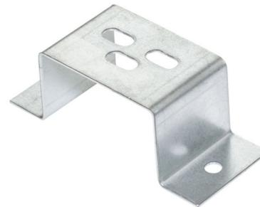
**Technical:****Product Type** Stand Off Bracket**Width** 50mm**Height** 40mm**Weight** 0.08 Kgs**Material** Pre-Galvanised Steel (Zinc Coated)**Colour/Finish** Self Colour**Standards** BS EN 10346:2015
