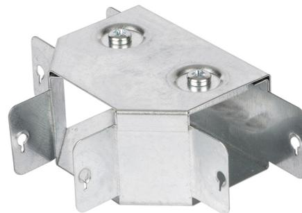
**Technical:****Product Type** Gusset Tee**Width** 50mm**Height** 50mm**Number of Compartments****Material** Pre-Galvanised Steel (Zinc Coated)**Colour/Finish** Self Colour**Standards** BS EN 50085-2-1 2006; BS EN 10346:2015
