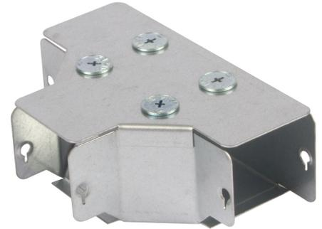
**Technical:****Product Type** Gusset Tee**Width** 50mm**Height** 50mm**Weight** 0.33 Kgs**Number of Compartments****Material** Pre-Galvanised Steel (Zinc Coated)**Colour/Finish** Self Colour**Standards** BS EN 50085-2-1 2006; BS EN 10346:2015**Trunking Weights:**
