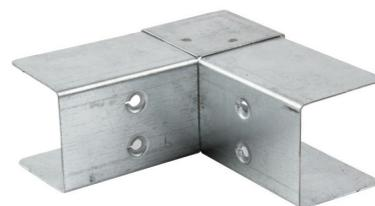
**Technical:****Product Type** Coupler**Width** 50mm**Height** 50mm**Weight** 0.23 Kgs**Angle** 90°**Material** Pre-Galvanised Steel (Zinc Coated)**Colour/Finish** Self Colour**Standards** BS EN 10346:2015
