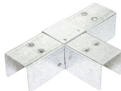
**Technical:****Product Type** Coupler**Width** 50mm**Height** 50mm**Weight** 0.35 Kgs**Angle** 90°**Material** Pre-Galvanised Steel (Zinc Coated)**Colour/Finish** Self Colour**Standards** BS EN 10346:2015**Important:**
