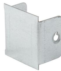
**Technical:****Product Type** Stop End**Width** 50mm**Height** 50mm**Weight** 0.02 Kgs**Material** Pre-Galvanised Steel (Zinc Coated)**Colour/Finish** Self Colour**Standards** BS EN 10346:2015**Important:**
