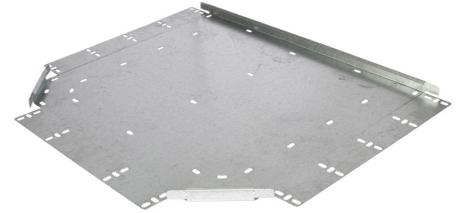
**Technical:****Product Type** Flat Tee**Width** 600mm**Height** 25mm**Weight** 4.83 Kgs**Gauge** Medium Duty**Material** Pre-Galvanised Steel (Zinc Coated)**Colour/Finish** Self Colour**Standards** BS EN 61537:2007; BS EN 10346:2015
