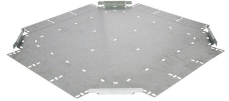
**Technical:****Product Type** Flat Fourway**Width** 600mm**Height** 25mm**Weight** 5.17 Kgs**Gauge** Medium Duty**Material** Zinc Magnesium Steel ZM310**Colour/Finish** Self Colour**Standards** BS EN 61537:2007; BS EN 10346:2015
