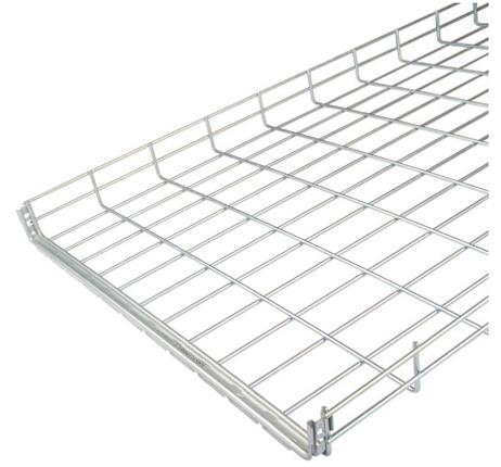
**Technical:****Product Type** Basket Tray**Width** 600mm**Height** 60mm**Length** 3000mm**Weight** 8.79 Kgs**Dimensions** 600 x 60mm mesh**Diameter** 4.8mm (Steel wire frame)**Outside Diameter** 4.8mm (Steel wire frame)**Material** Electro Zinc (E.Z)**Colour/Finish** Self Colour**Standards** BS EN 61537:2007**Supplied With** Pre-Installed FastConnect Coupler
