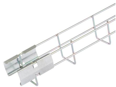
**Technical:****Product Type** Basket Tray**Width** 60mm**Height** 60mm**Length** 3000mm**Weight** 1.41 Kgs**Dimensions** 60 x 60mm mesh**Diameter** 3.9mm (Steel wire frame)**Outside Diameter** 3.9mm (Steel wire frame)**Material** Electro Zinc (E.Z)**Colour/Finish** Self Colour**Standards** BS EN 61537:2007**Supplied With** Pre-Installed BT/FX60 Couplers
