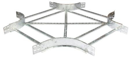
**Technical:****Product Type** Fourway**Width** 750mm**Height** 125mm**Weight** 18.00 Kgs**Diameter** 300mm Radius**Gauge** 1.5mm**Material** Post Hot-Dipped Galvanised (HDG)**Colour/Finish** Self Colour**Standards** BS EN ISO 1461:2009**Important:**
